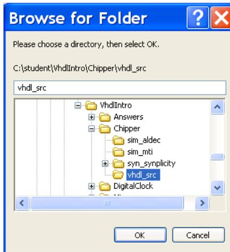
Note if a simulation is active, you cannot run change directory. First you must end the simulation with the ModelSim menu pull down "Simulate > End Simulation".
